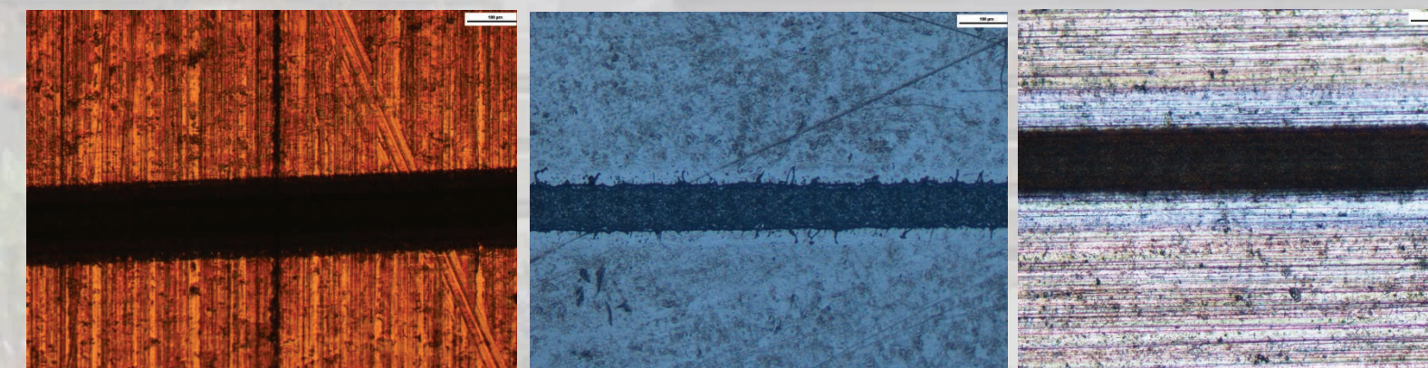
pulse -35 fs, \lambda = 800 nm, cutting speed 10 mm/s
